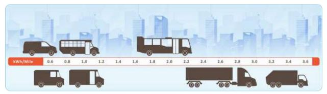
Figure 5: Typical BEV energy consumption rates for medium- and heavy- duty vehicles.
