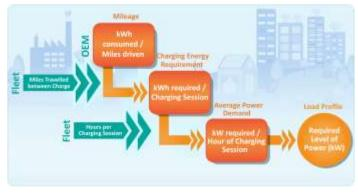
profile is straightforward, provided that you Figure 4: Components and process for developing your load profile
