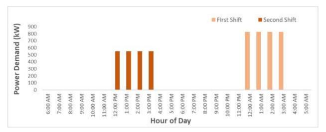
Second Shift Average Power Demand (kW) = 2,200 kWh / 4 hours = 550 kW
